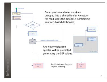
This is a breakdown of the processing done to set up the SQL database and the visualizations seen during the loading of data. Once built, any new data is shipped to the on-line viz but also predicted using the most recently-generated model. This tells us when a model requires updating.
