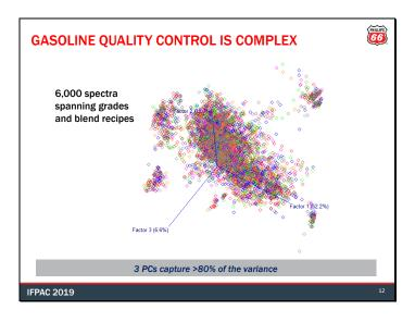
Gasoline blending is necessarily a dynamic process. This PCA plot, where each point represents the spectrum of a unique point in time, displays both the trends and the clustering of the data that is related to blend recipe and grade. The structure is there; we need to ensure we can make the most of the calibration opportunity.
