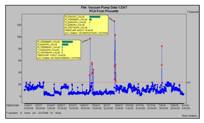
Figure 8. Quality Analyst deployment of multivariate model for vacuum pumps
