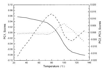
FIG. 3. Score plots vs. temperature for the temperature-dependent FT-IR spectra of an LB film of PtBMA. Solid, dashed, and dotted lines represent the PC1, PC2, and PC3 scores, respectively.
