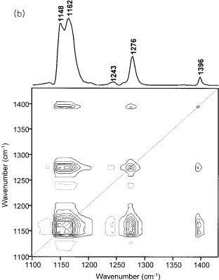
Fig. 5. Synchronous 2D correlation and power spectra of the LB film of PtBMA (a) below the glass transition temperature (26–66 °C) and (b) above the glass transition temperature (93–136 °C). Solid and dashed lines represent positive and negative cross peaks, respectively.
