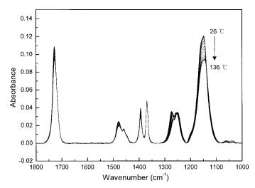
Fig. 1. Reflection absorption FT-IR spectra of a 50-layer LB film of PtBMA at various temperatures (26–136  $^{\circ}{\rm C}$ ).
