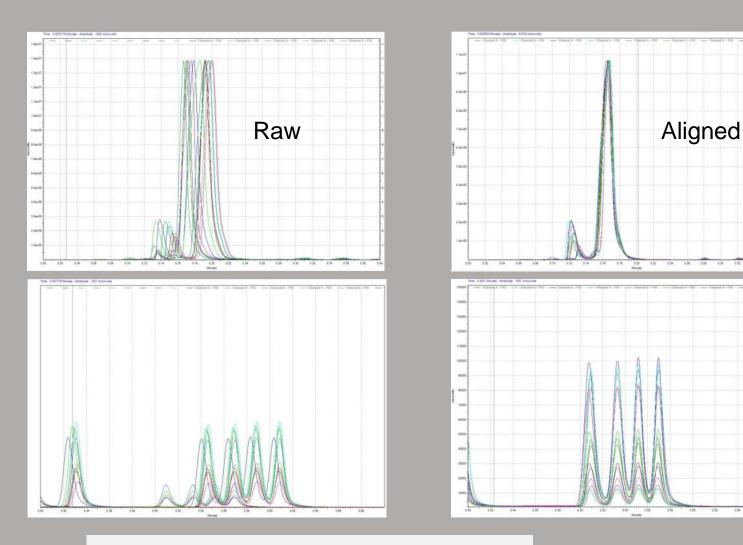
Two instruments with nominally the same method and columns, manual injection
