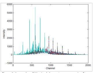
Figure 1. An overlay of 11 mixed chromatograms ranging from pure kerosene to pure diesel
